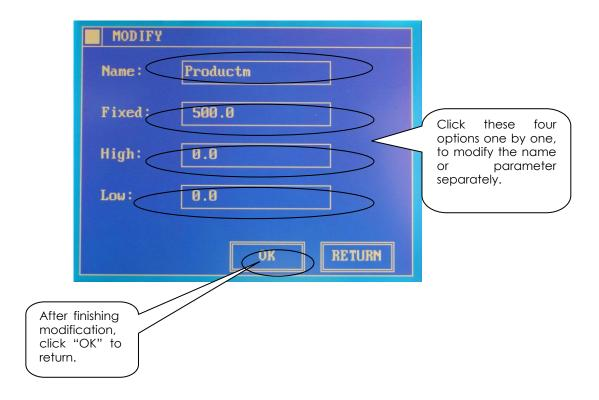
The function of product editing is to meet the customer"s requirement of testing different products. After being set, the same product can be directly loaded in the next time, that is to say, once and for all.
